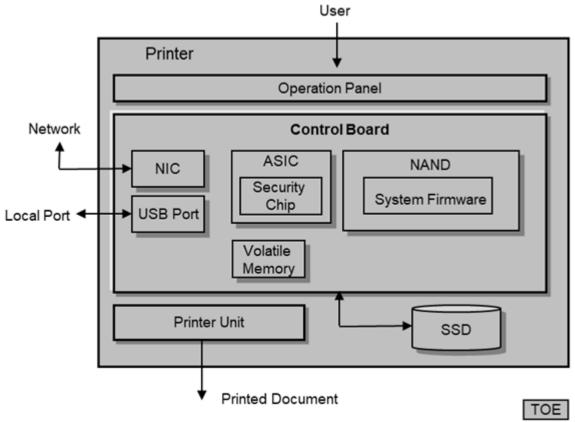
Figure 1. Physical configuration of the TOE
